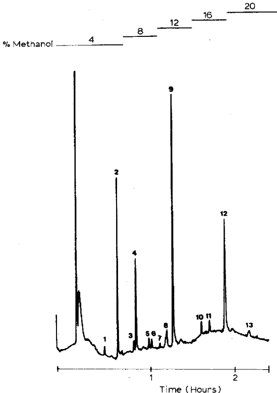
Fig. 2. Separation of the major and minor nucleosides from the hydrolysis of 100 ng of tRNA-Phe. The gradient is the same as in Fig. 1. Elution order: (1) pseudouridine, (2) cytidine, (3) 5-methylcytidine, (4) uridine, (5) 5-methylguanosine, (6) 2'-O-methylcytidine, (7) 5-methyluridine, (8) 1-methyladenosine, (9) adenosine, (10) 2'-O-methylguanosine, (11) \text{N}^2 -methylguanosine, (12) guanosine, (13) \text{N}^2, \text{N}^2 -dimethylguanosine.
